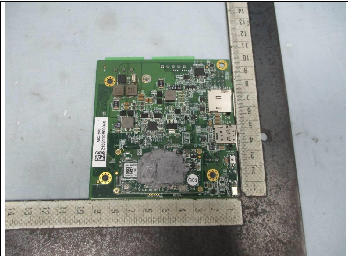
Bottom side view of RTC battery board
