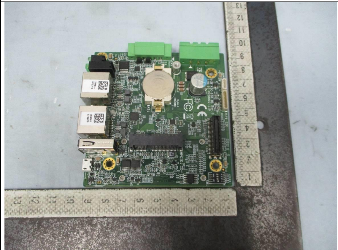
Top side view of RTC battery board
